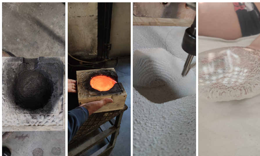
Fig. 2. Image of the 3D-printed mold, the field test at the Lavai kiln, the construction of milling molds, and the results of their use. Photos: D. Rolli, D. Crippa, et al.
