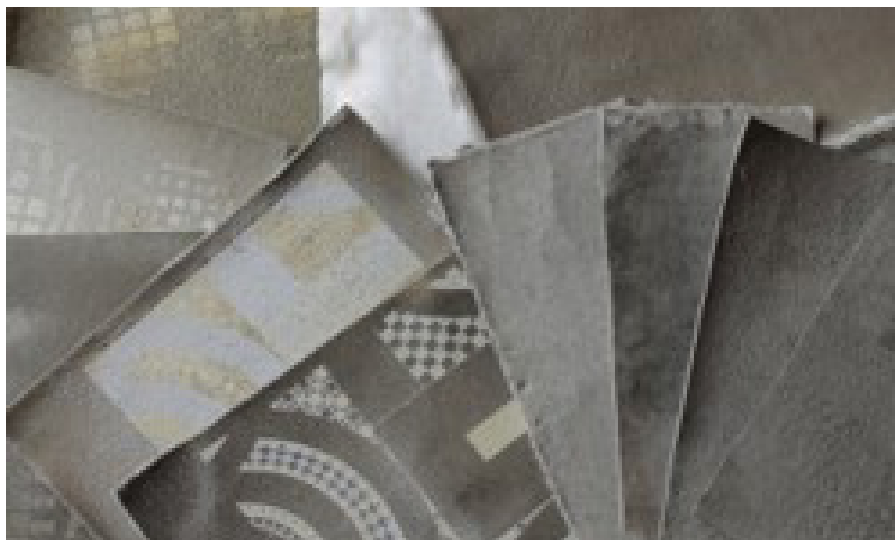
Fig. 6. Lithos – A composite bio-leather developed from waste basalt and Roman travertine powders embedded in biopolymer matrices, which can be applied to textile substrates using coating and casting techniques.
