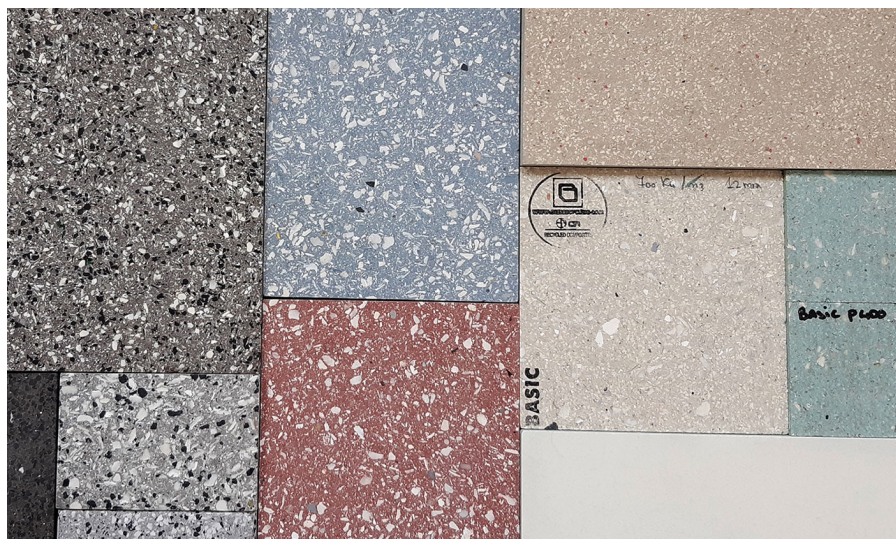
Fig. 2. Panels made from recycled composites. Photo: Gees Recycling
